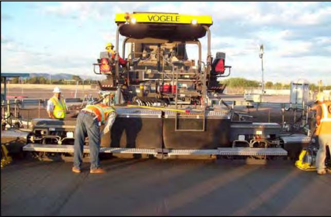
**Figure 8.** High-density RCC paver.
