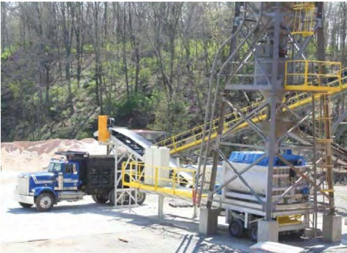
**Figure 6.** Twin shaft horizontal mixer—batch type.
