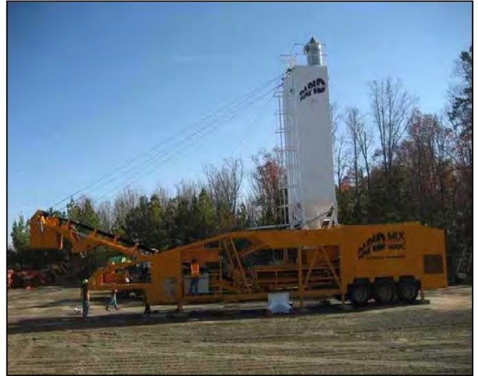
**Figure 7.** Twin shaft horizontal mixer—continuous type.
